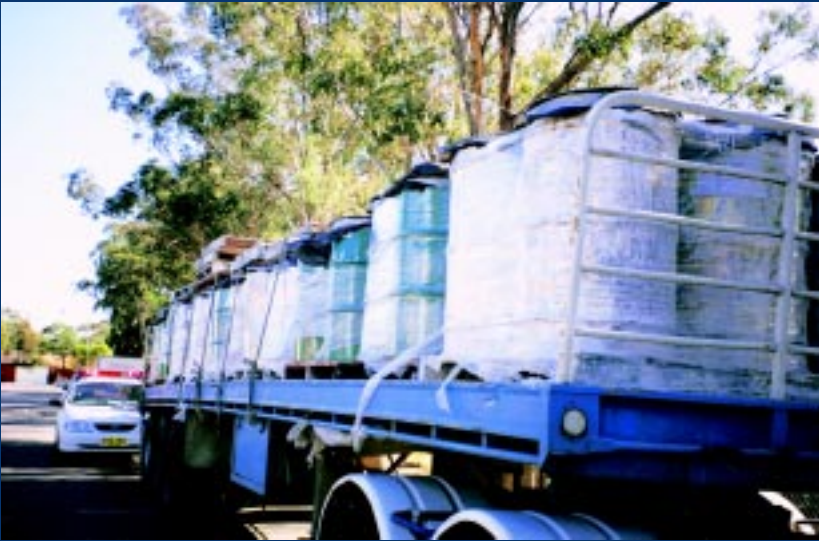
Some of these drums were unrestrained and others that were tied down with rope, did not meet the minimum restraint requirements (see page 66).
