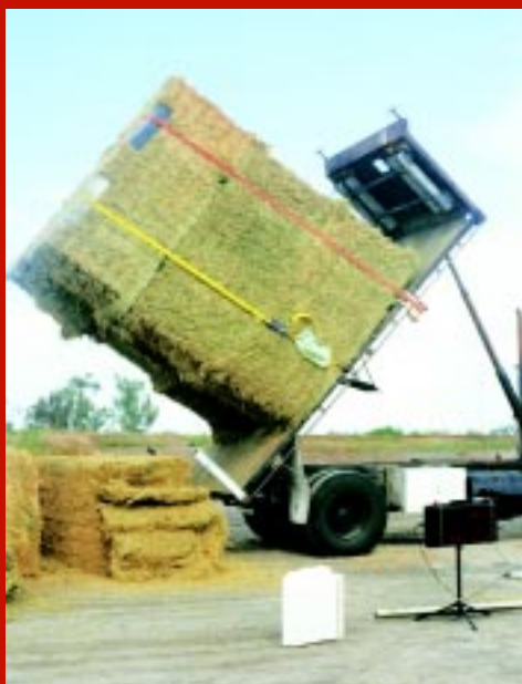
Load testing large hay bales (2.4 m x 1.2 m x 1.2 m). In this case only one webbing strap per row was used and the bales collapsed.
