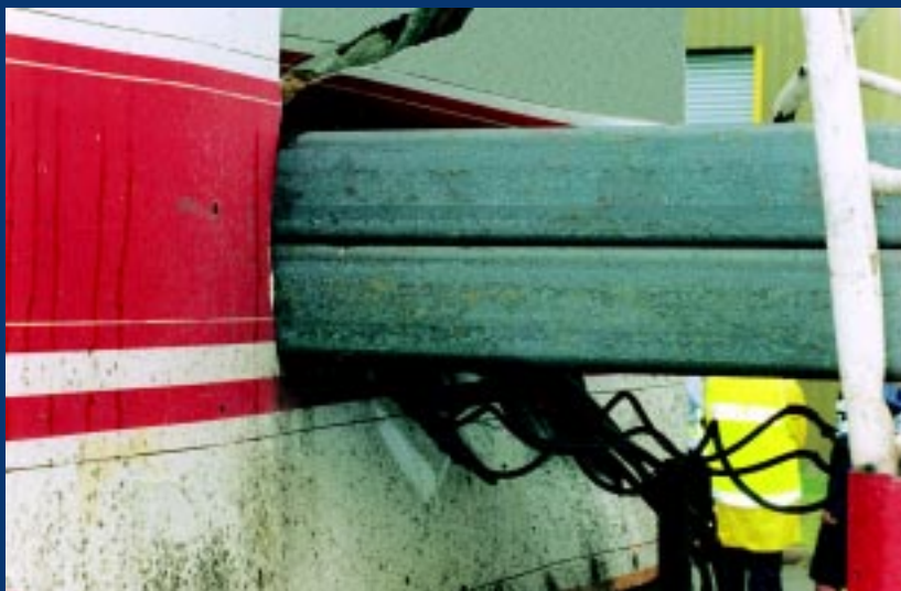
12 steel billets weighing 24 tonnes in all, pierced the cab of this truck. Note that the pipe loading rack (far right) was ineffective.
