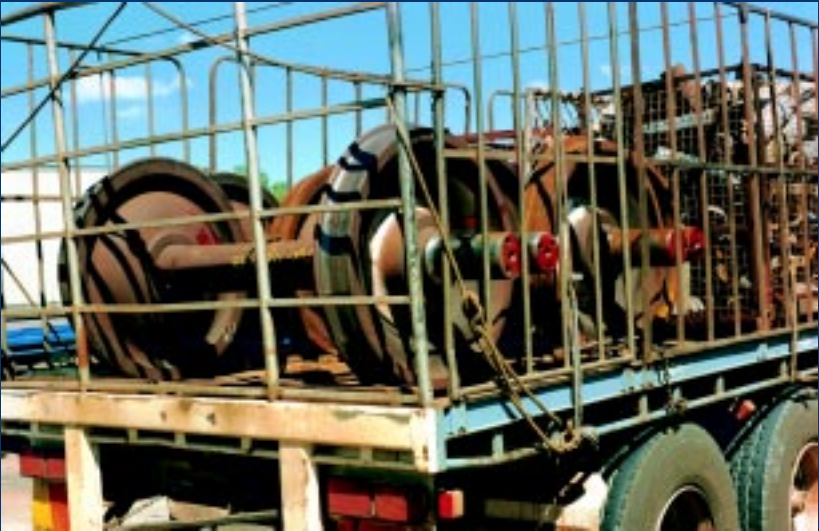
The loading rack and its support rope will not restrain these rail wheels and axles.
