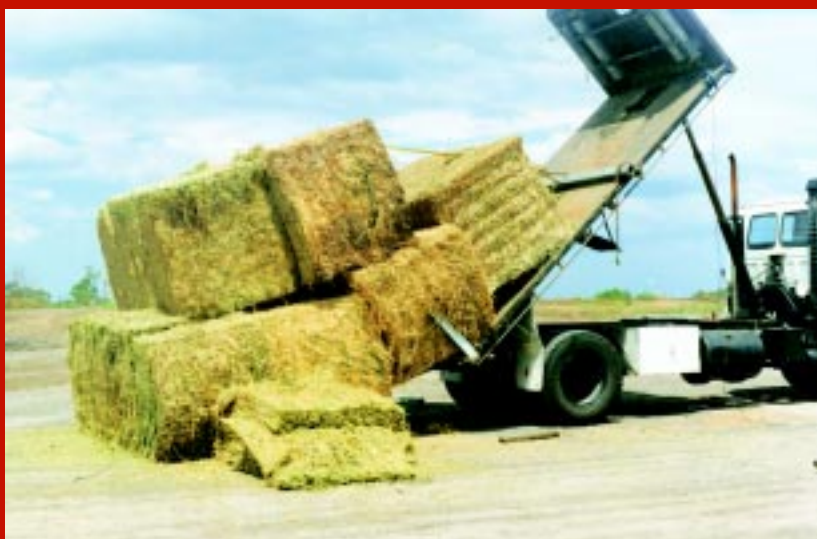
Load testing large hay bales (2.4 m x 1.2 m x 1.2 m). In this case only one webbing strap per row was used and the bales collapsed.
