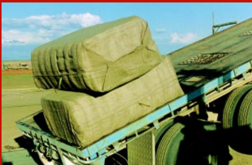
Testing the friction by tilting the load and measuring the angle at the point it just slides. The test is for both the friction between the bales and the bales and the deck.
